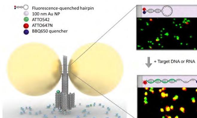
**Figure 1.** Illustration of fluorescence-quenched hairpin assay incorporated in the hotspot of plasmonic gold dimer nanoantenna: upon binding of the target DNA/RNA target fluorescence enhancements of ATTO647N reaching several hundred fold can be achieved.
