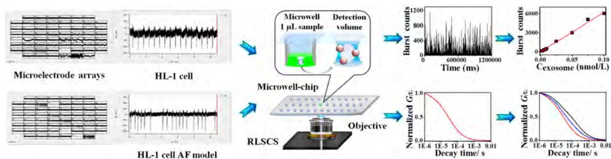
**Figure.** The principle of determination of AF related exosomes by MC-RLSCS.
