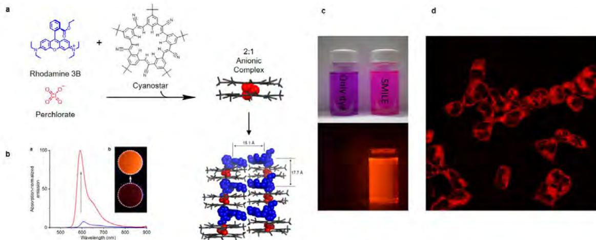
**Figure.** (a) Supramolecular assembly of SMILES crystals, decoupling the dyes. (b) Fluorescence from rhodamine thin film with and without cyanostar. (c) 20 nm ligand stabilized rhodamine SMILES nanoparticles in water. (d) HeLa cells stained with SMILES nanoparticles.
