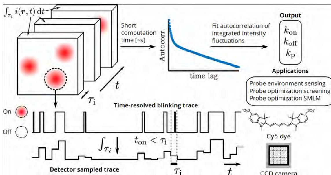
**Figure.** Overview of image correlation based method for rapid measurement of fluorophore blinking rate constants
