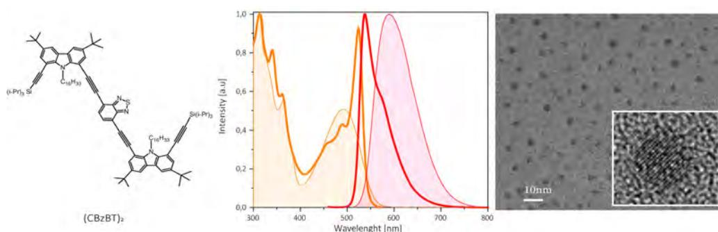
**Figure.** (left) Chemical structure of (CBzBT)<sub>2</sub>. (center) Absorption (orange) and fluorescence (red) spectra of (CBzBT)<sub>2</sub>. The filled and solid lines are the spectra of (CBzBT)<sub>2</sub> in THF and the organic nanodots (ONDs) dispersed in water, respectively. (right) TEM micrograph showing spherical morphology of the ONDs. The inset show a HR-TEM of a single OND, which reveals a quasi-crystalline diffraction pattern with lattice fringes.
