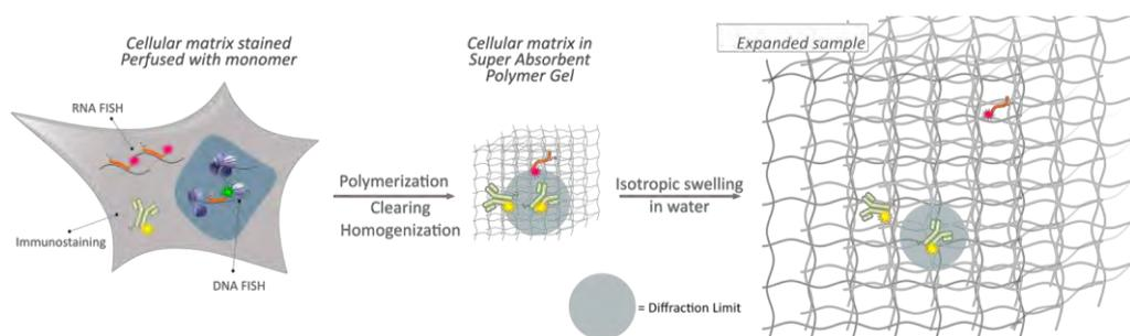
**Figure.** Different biomolecules of interest (DNA, RNA, proteins) can be cross-linked into a super-absorbent polymer followed by isotropic expansion to improve resolution.
