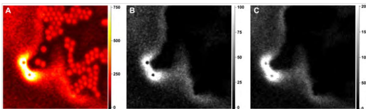
**Figure 1.** Anti-Stokes fluorescence microscopy, using optically activated delayed fluorescence (OADF) and upconversion fluorescence (UCF). A) Normal fluorescence image, B) OADF image, C) UCF image. Image taken from Reference 1.
