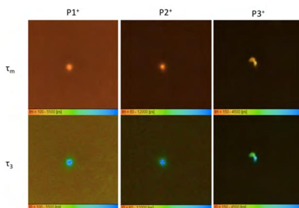
**Figure.** Time-resolved fluorescence images of three conjugated polyelectrolyte samples represented as: (i) average fluorescence lifetime,  $\tau_m$ , maps and (ii) the  $\tau_3$  component, after extended periods of focussed, IR laser irradiation.
