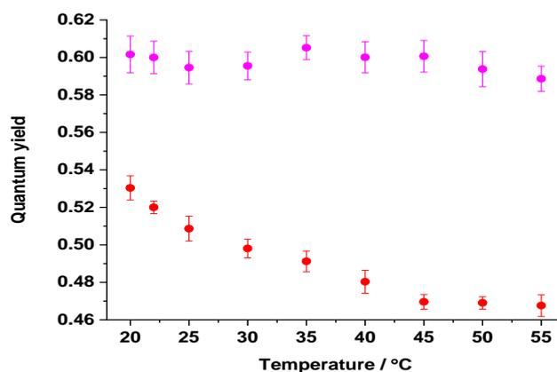
**Figure.** The quantum yields of quinine in 0.05M sulfuric acid (red) and in 0.1M perchloric acid (magenta).
