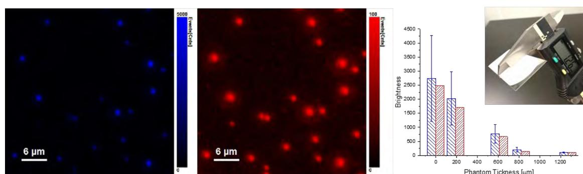
**Figure.** Single particle-images of SWIR-emitting Pdots deposited on tissue-mimicking phantom recorded simultaneously by Si detector (blue) and InGaAs detector (Red) together with diagram of particle brightness for different phantom thickness.
