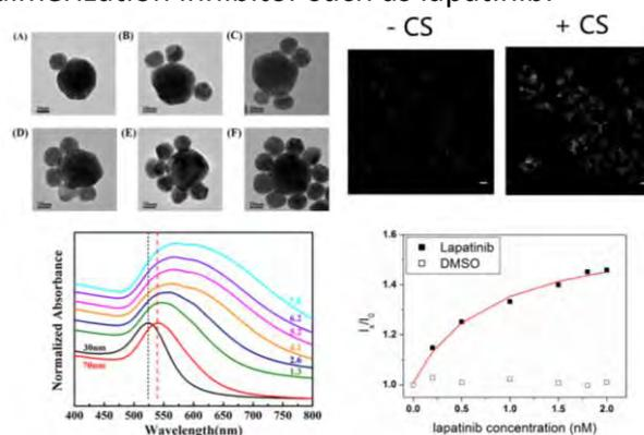
**Figure.** TEM image of different CS nanostructure, absorption spectra, the enhanced fluorescence images of HeLa cell with CS, and the dependence of fluorescence intensity on dimerization inhibitor –lapatinib.
