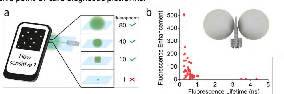
**Figure:** **a)** Representation of the sensitivity of modern smartphone cameras tested with ATTO542 fluorescent dye DNA origami beads. **b)** Fluorescence enhancement of ATTO647N achieved in the hotspot of a DNA origami-based nanoantenna employing 80 nm silver nanoparticles.
