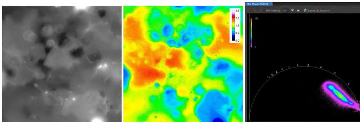
**Figure 1.** From left to right: fluorescence image of a filter paper with a variety of dust and microplastic particles, phase angle based fluorescence lifetime distribution in the range of 0.6 ns – 2.9 ns, the corresponding phasor plot.
