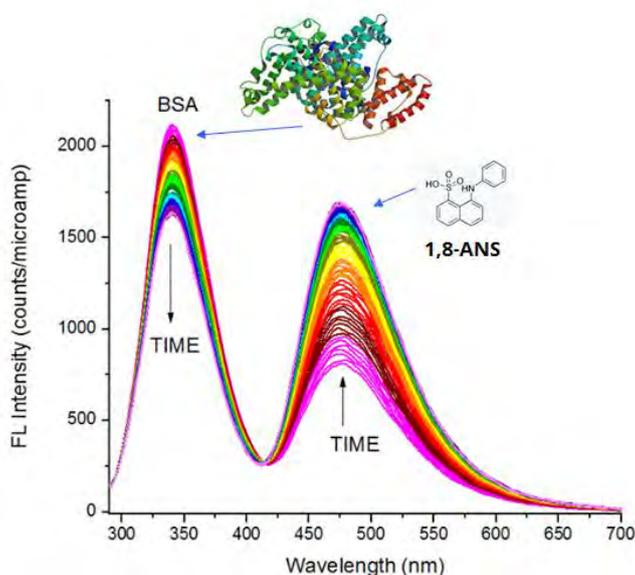
**Figure.** Fluorescence Spectral Kinetics of binding and energy transfer from BSA protein to 1,8-ANS. Structure of BSA.<sup>1</sup>
