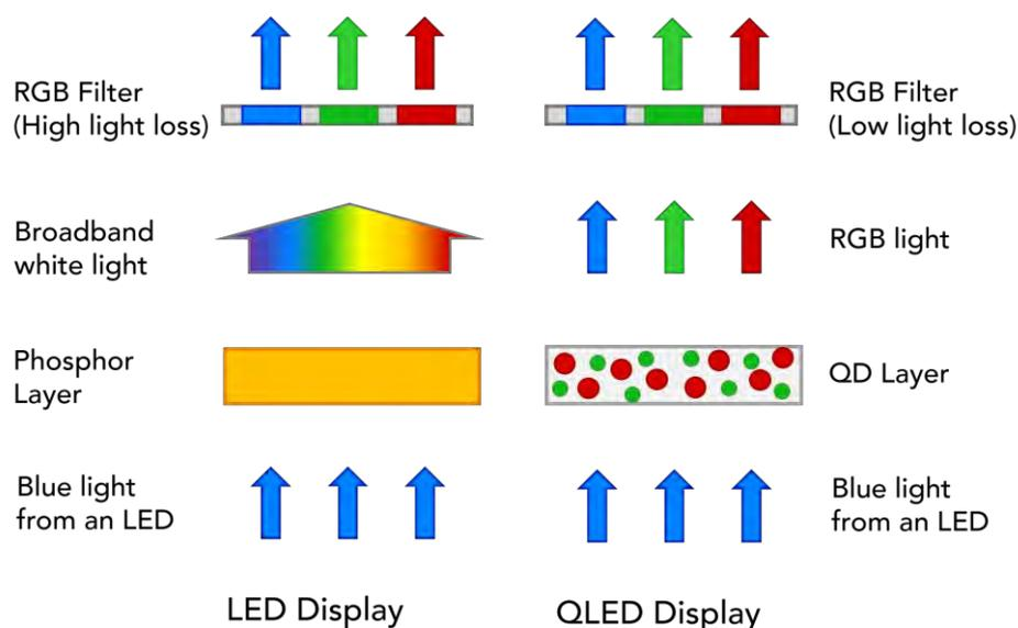
**Figure.** Operating principle of LED & QLED displays.
